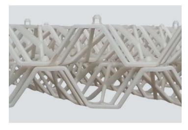
BESE-Elements® grids feature a patented push button connection, thus single layers can be combined to solid blocks. These blocks can be used as single blocks or, with a certain offset, can be fixed together to form endless blocks.
