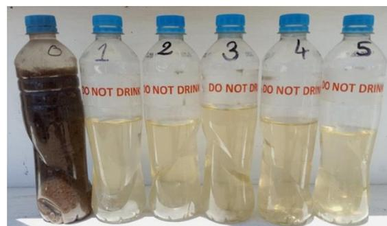
Figure 2: Sludge filtrate (sampled every 15min after loading). Sludge sample (0) included as reference
