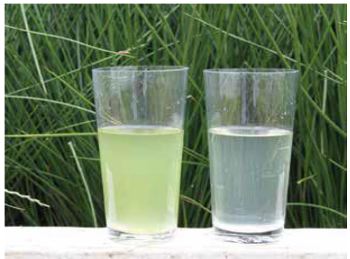
Wetland influent (left – SS>150mg/L) versus effluent (right – SS<10mg/L)
