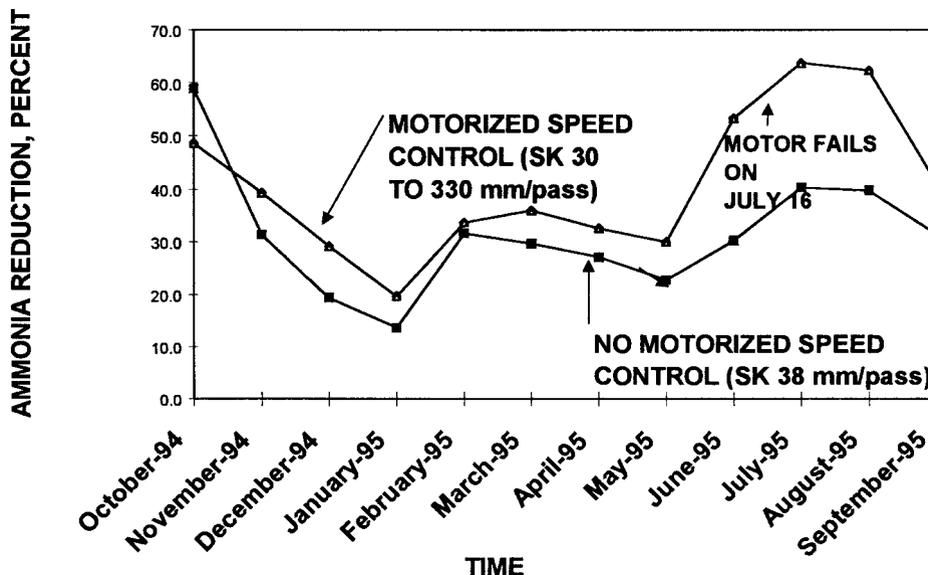
**FIG. 2. Ammonia Reduction at Central Valley As Function of Distributor Speed Control**
