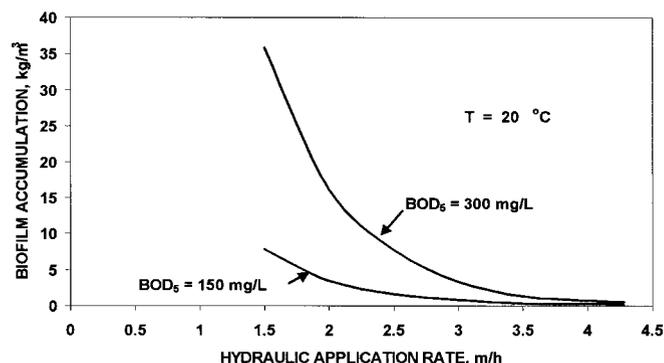
**FIG. 3. Solids Accumulation in XF Media As Function of Application Rate and BOD (Battistoni et al. 1992)**
