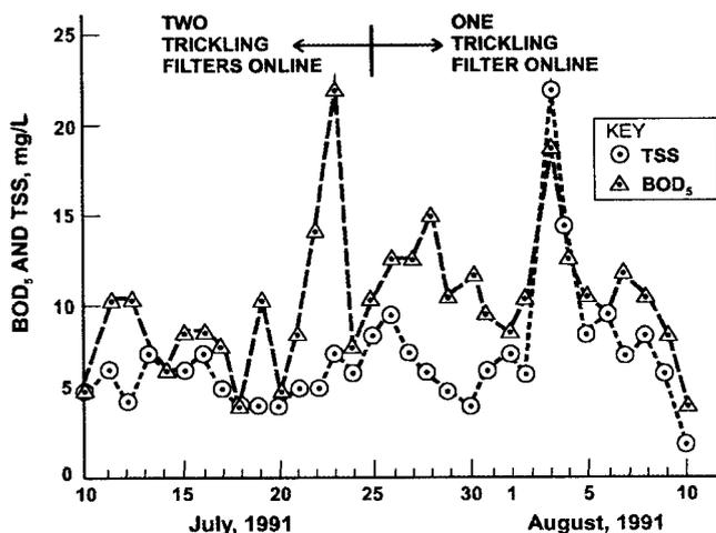
FIG. 1. Effect of Shock Loading on TF/SC Process at Omaha
